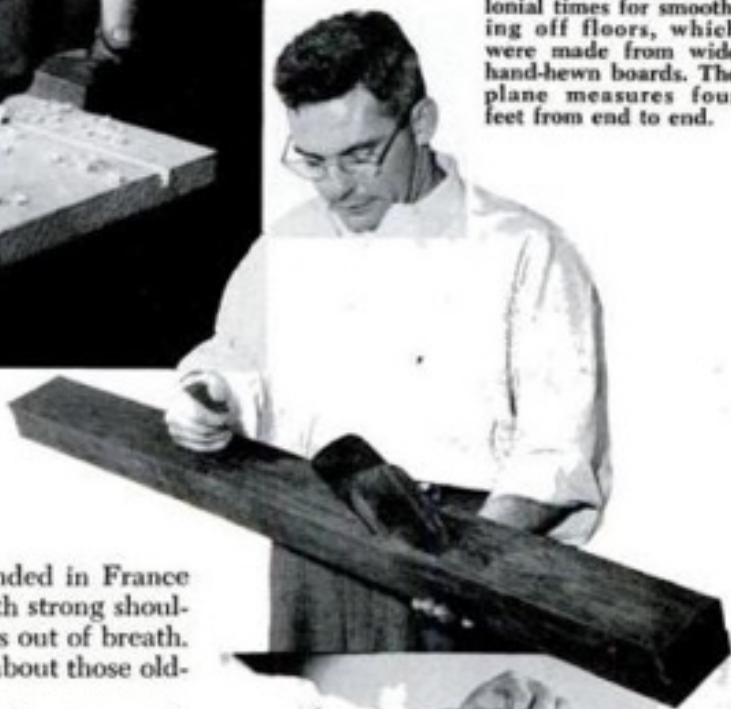
PLOW PLANE with wood screws (above) was made from boxwood by an early American toolmaker. It still cuts a clean dado. Fence and blade are adjustable.
