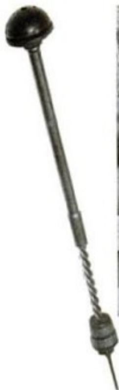
THIS HUGE "PUMP-LOG" AUGER was used for boring 1½-inch (inside diameter) pipes from wooden logs. Zlotoff found it in the dusty rafters of an old farm-implement shed and discovered that although it was rusty it still worked. Here he bores into a maple log; the handle is offset to provide leverage needed to turn this heavy tool. At the left is an early push-drill which is still in good operating condition.
