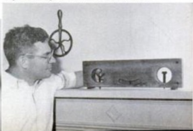
OLD-TIME LEVEL has no bubble, but a bob-like pointer. Screw feet adjust level to any angle. Measuring wheel (on wall) did a job that steel tapes do today. This one is two feet around.
