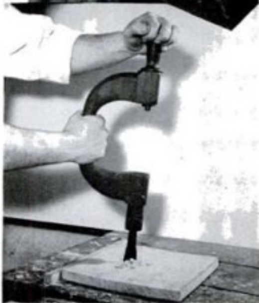
THERE'S NO CHUCK on this brace and bit, which dates back to early colonial America. This style was in use in Europe more than 500 years ago. It uses a center bit rather than a spiral bit.
