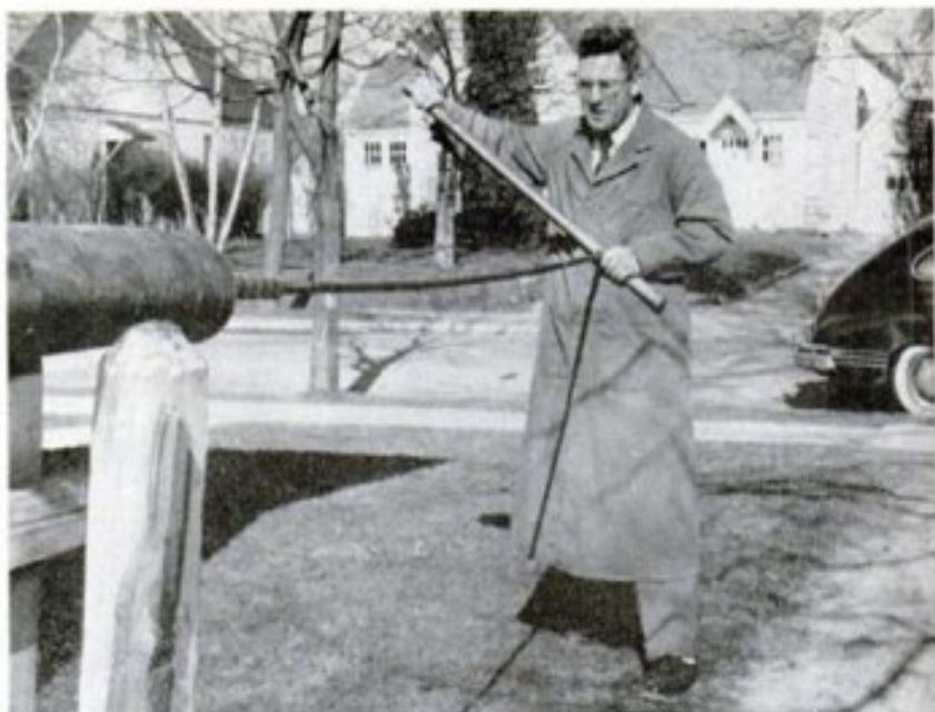
THIS HUGE "PUMP-LOG" AUGER was used for boring 1½-inch (inside diameter) pipes from wooden logs. Zlotoff found it in the dusty rafters of an old farm-implement shed and discovered that although it was rusty it still worked. Here he bores into a maple log; the handle is offset to provide leverage needed to turn this heavy tool. At the left is an early push-drill which is still in good operating condition.
