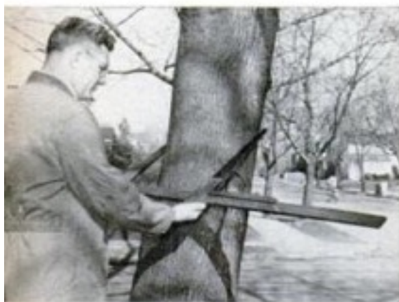
OLD LOGGER'S CALIPERS have a sliding wooden scale that tells at a glance how many board feet are in a log. Zlotoff found them among some old tools in an eastern Massachusetts shop.
